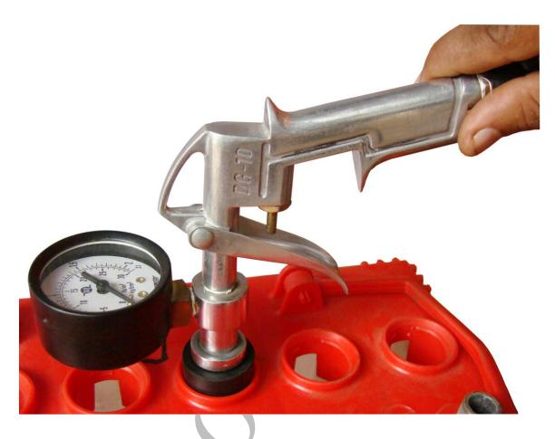
d. There may be leakage cell to cell leakage but not from sealing, it can be from welded L connection at partition.
