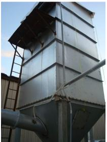
axially air taint with proper fitments. One ID blower fan of proper suction of air with control dampers. Bag house will be fitted with motorized rotary valve, scrubber with as per pollution board parameters (made by M. S. sheet, S. S. optional). One Chimney with base plate and monkey ladder up to pollution check point. One pollution checking deck and proper sampling port.
