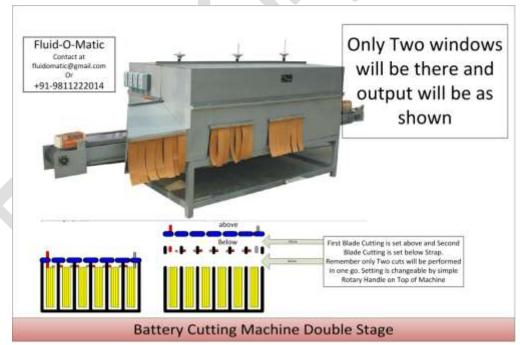
This machine is suitable for normal quantity of Batteries or by small smelter with normal budget. Power required: 415V 3 phase, 8 Kw approx.
