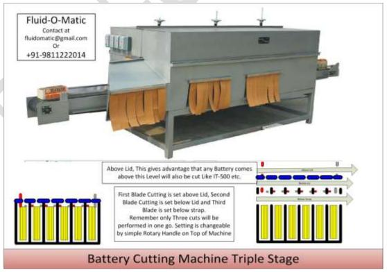
This machine is suitable for normal quantity of Batteries or by small smelter with normal budget. Power required: 415V 3 phase, 12 Kw approx.
