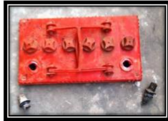
EXTRACTED POLES FROM BATTERY COVER
