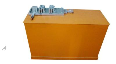
So these will depends on no. of sizes Batteries, you want make. Function of Comb Sets: Plates are brazed together in pack to make parallel circuit of many plates. No. of plates will determine capacity of Cell to supply current in ampere.
