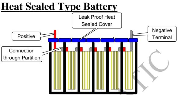
Advantages to manufacture Battery by Heat Sealing Process Method:
