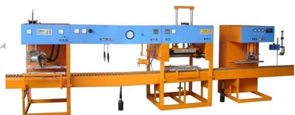
Machine melts lid & container simultaneously & presses to seal together and form a single identity so acid does not leak out. This saves Labour cost and cost of adhesive material. In turn it reduces inventory cost which will be inherited when battery is holded for drying period and labour is involved in drying process.
