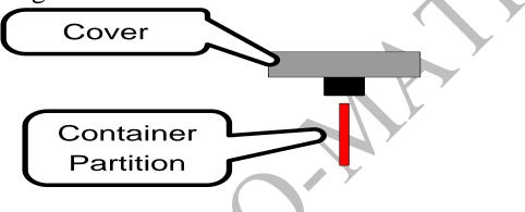
If this is not done, it will result in leakage. Best Heat Sealing is done in homogeneous material. If materials are different for cover & container then also it will leak at later stage. How exactly it all functions this follows: Cover from battery is picked up by the top fixture either by vacuum or by hooks.
